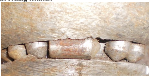
Fig. 1 Appearance of worn rollers of the bearing assembly after operation
