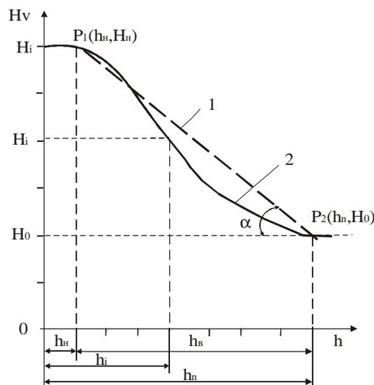
**Fig. 1 – Distribution of hardness through the thickness of the nitrided layer:
