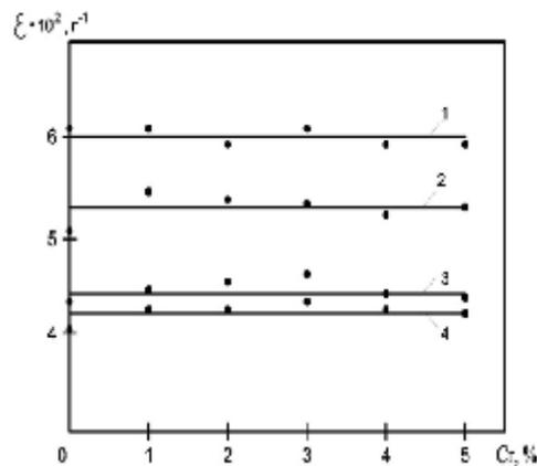
**Fig. 1 – The dependence of the wear resistance  $\varepsilon$  of steel on the content therein chromium Cr for temperature tempering: 1 – 373K; 2 – 473 K; 3 – 673 K; 4 – 873 K**
