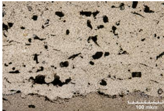
Fig. 9. Microstructure of the Ni-Cr-B-Si system coating
