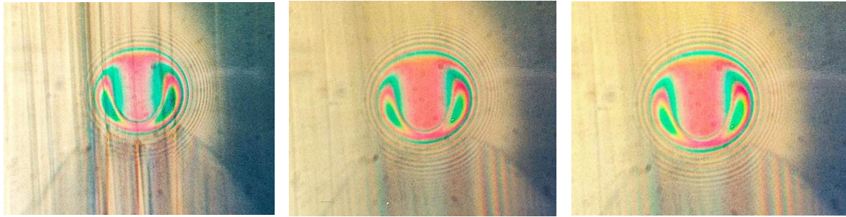
Fig. 8. Selection of micro-interferograms for a point EHD contact ( R_y/R_x = 1 ) across a range of contact loads F from 7.78 to 46.68 N (the SAE 75W-90 transmission oil)
