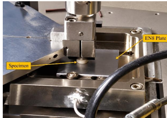
Fig 3. Linear Reciprocating Tribometer: Specimen & EN8 Plate
