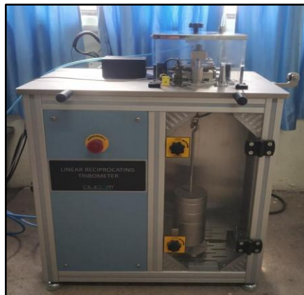
Fig 2: Schematic Linear Reciprocating Tribometer
