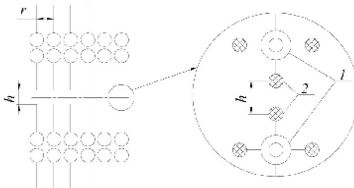
Fig.1 – Molecular arrangement of fatty acid in smectic boundary layer:
