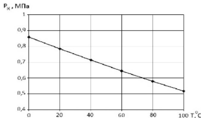
Fig. 7 – Change in specific cohesion force depending on temperature
