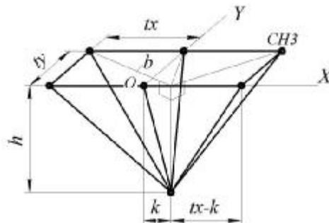
**Fig. 5 – Design diagram for determination of cohesion force**
