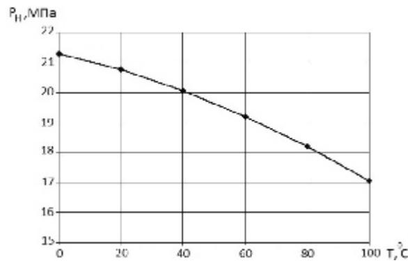
**Fig.4 – Change in layer bearing capacity depending on temperature**
