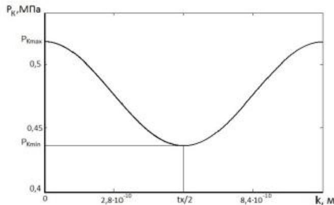
Fig. 6 – Change in specific cohesion force in relative shift of smectic layers
