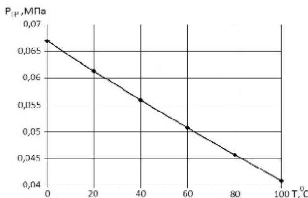
**Fig. 8 – Changes in specific friction force in layers of smectic liquid crystal**
