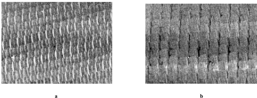
**Fig. 3 – Surface structures after milling and turning with various parameters:**
