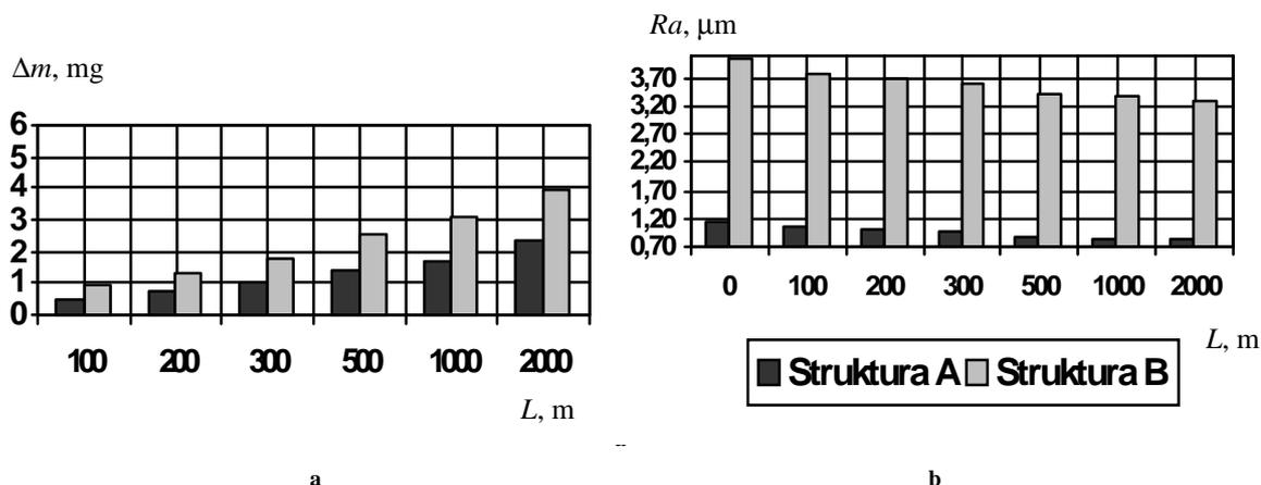
Fig. 5 – Change in the surface layer condition for samples after EDM treatment as a function of the path of friction, denoted by:
