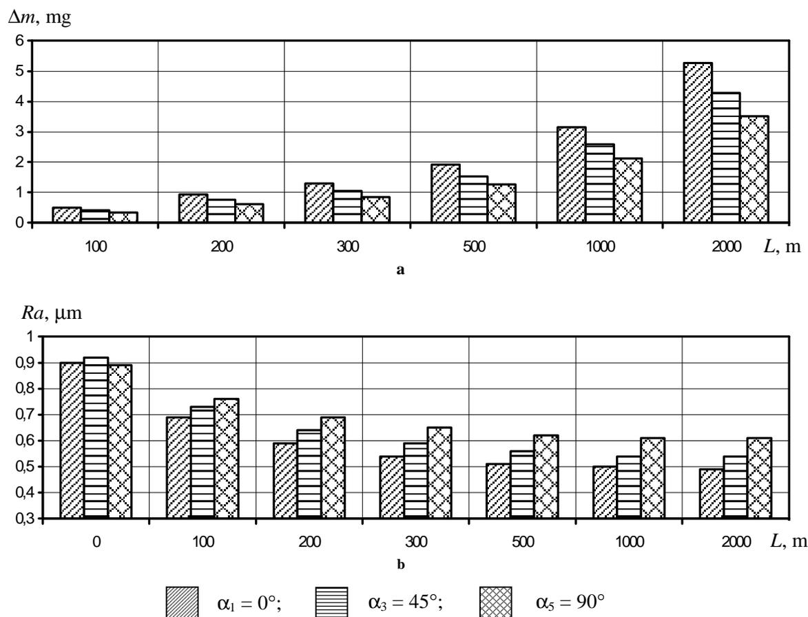
Fig. 4 – Change in the surface layer condition for ground samples as a function of the path of friction, denoted by:
