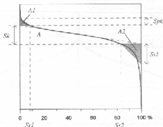
Fig. 2 – Characteristics of bearing curve [5]
