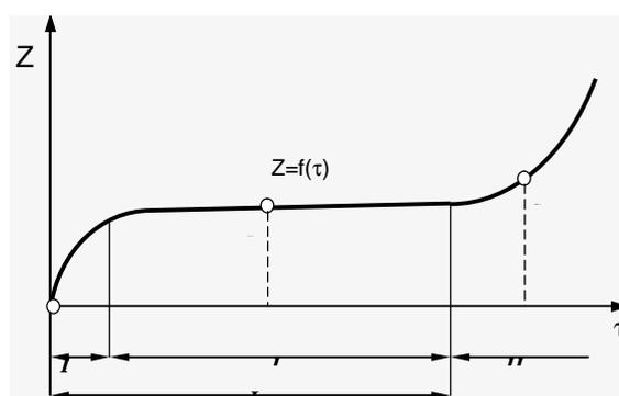
Fig. 1 – Graphic record of a typical wear process
