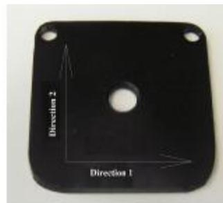
Fig. 5 – Examined sample coated with CROMVIC<sup>2</sup>
