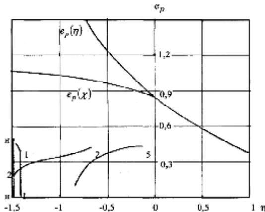
Fig. 1 – Chart plasticity of steel 20X and ways of deformation dangerous areas during the introducing of splined stamp
