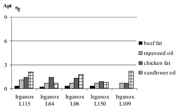
Fig. 9 – Oxidation susceptibility of fats with various antioxidants calculated in terms of change in viscosity depending on temperature ( $\dot{\gamma} = 1333 \text{ s}^{-1}$ ), calculation point is 50 °C
