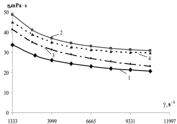
**Fig. 2 – Dependence of viscosity on the shear rate (at 50 °C) for animal fat:**
