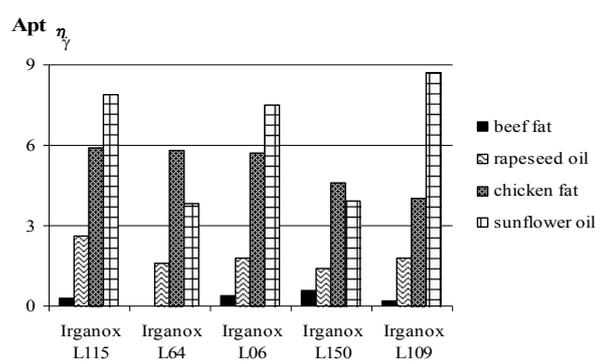
Fig. 10 – Oxidation susceptibility of fats with various antioxidants calculated in terms of change in viscosity depending on shear rate ( $t = 50 \text{ °C}$ ), calculation point is  $10667 \text{ s}^{-1}$
