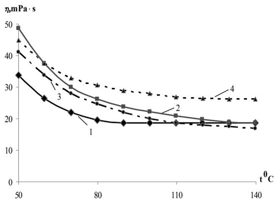
**Fig. 1 – Dependence of viscosity on temperature (at  $\dot{\gamma} = 1300 s^{-1}$ ) for animal fat:**
