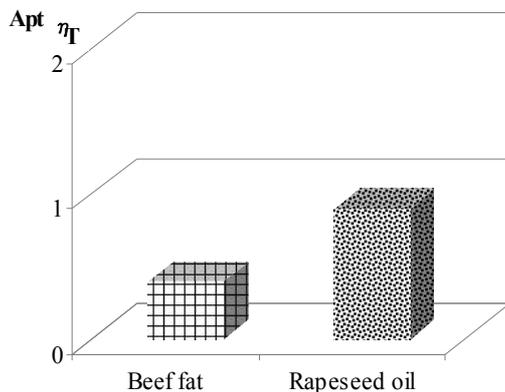
Fig. 5 – Oxidation susceptibility of fats calculated in terms of change in viscosity depending on temperature ( $\dot{\gamma} = 1333 \text{ s}^{-1}$ ), calculation point is 50 °C
