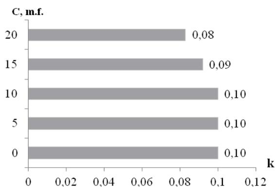
Fig. 6 – Friction coefficient for the developed lubricant with different concentrations of P400 paraffin
