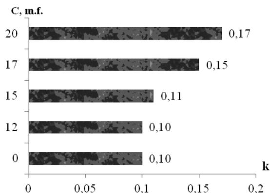
Fig. 9 – Friction coefficient for the developed lubricant with different concentrations of concentrations of bentonite
