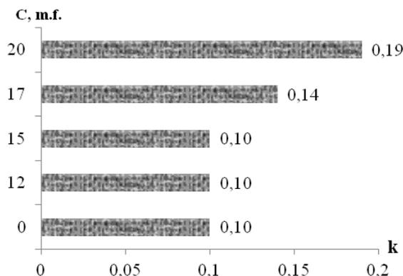
Fig. 8 – Friction coefficient for the developed lubricant with different concentrations of aerosil 200
