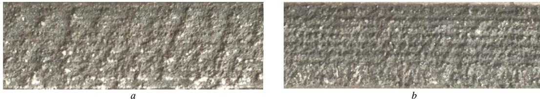
Fig. 1. General view the surface of the laser modified SiC carbide layer on the alloy 7075 with a coefficient of overlap of the laser tracks 25% (a) and 50% (b),  $\times 25$
