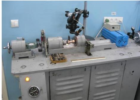
Fig. 2. General view of the operating unit of the friction machine MFC-1
