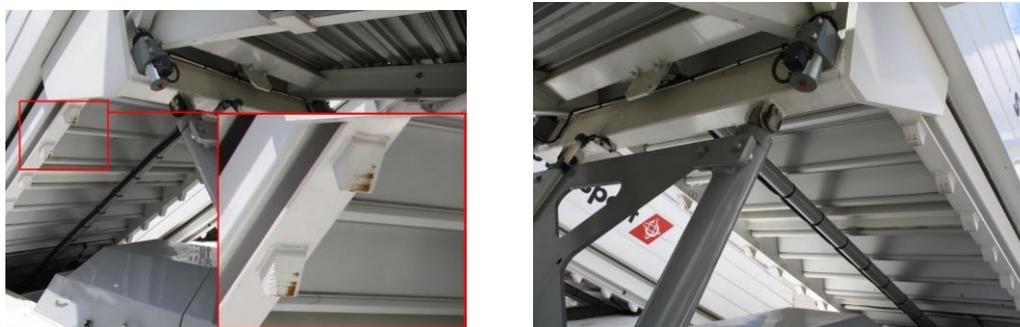
**Fig. 1. The result of excessive wear of the supporting teeth in the locking section of the self-propelled passenger stairs ABS 580 firm TLD:**
