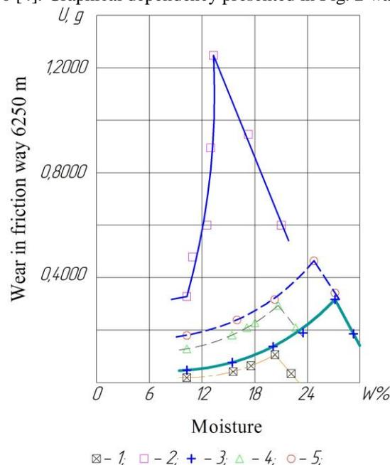
**Fig. 2. Dependence of wearability of soils on moisture:**
