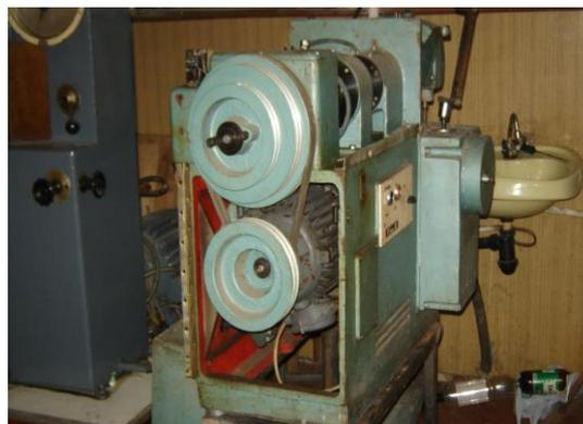
**Fig.4 Friction machine SMC-2**
