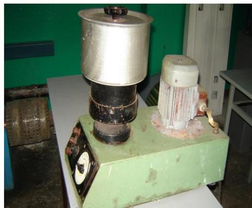
**Fig.2. Mill MPR-2 :Technical characteristics: Productivity, samples / hour - 10; Grinding time of one sample, min-3; Mass of samples, Mr -100; Voltage, at 380; Power, kW - 0.6; Speed, rpm -7000**
