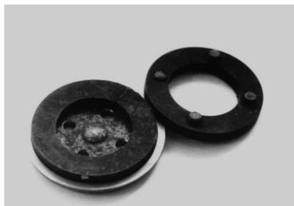
**Fig.13. Billets for the thrust of the electric motor of the pump.**
