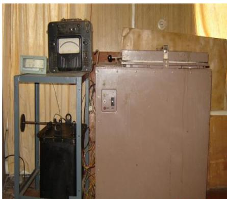
**Fig.3 Electric furnace SSHO-3, Technical characteristics: Voltage, at 220; Power, kW- 6; Nominal temperature,  $^{\circ}\text{C}$  - 380**
