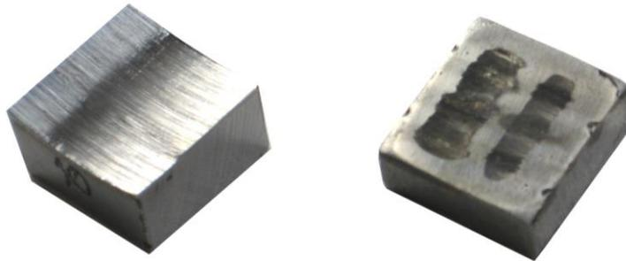
Fig. 4. Samples from a CEC after friction test
