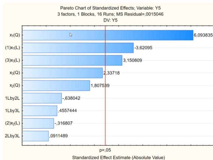
Fig. 5. Standardized Pareto map for surface roughness  $R_a/R_{a\text{init}}$
