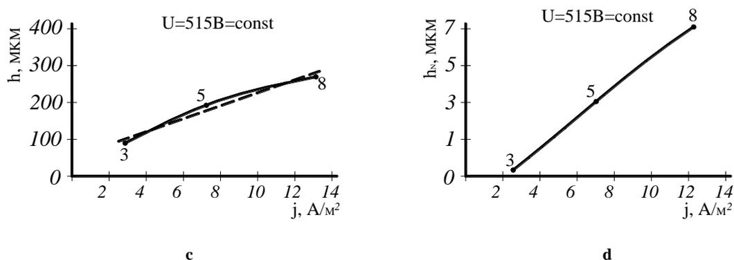
**Fig. 8 Dependences of the depth of the diffusion layer  $h$  (a) and the nitride layer  $hN$  (b) on the voltage at  $j = 7.2 \text{ A/m}^2 = \text{const}$ ; also c and d on the current density  $j$  at  $U = 515B = \text{const}$**
