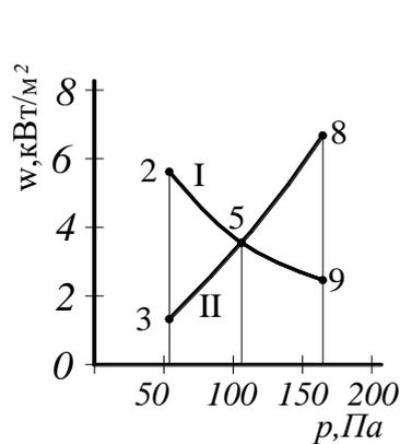
**Fig. 6. Dependence of the specific power  $w$  on the pressure of the gas mixture  $p$  at BATR with autonomous saturation modes (curve I – nitriding at  $U = 515$  B = const and curve II – nitriding at  $j = 7.2$  A / m<sup>2</sup> = const)**
