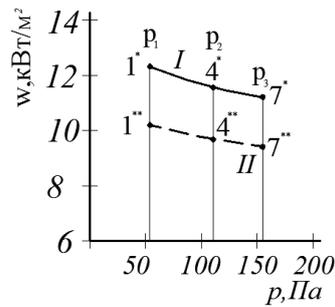
**Fig. 3. Dependences of the specific power of the discharge  $w$  on the pressure of the gas mixture at interdependent BATR modes:**
