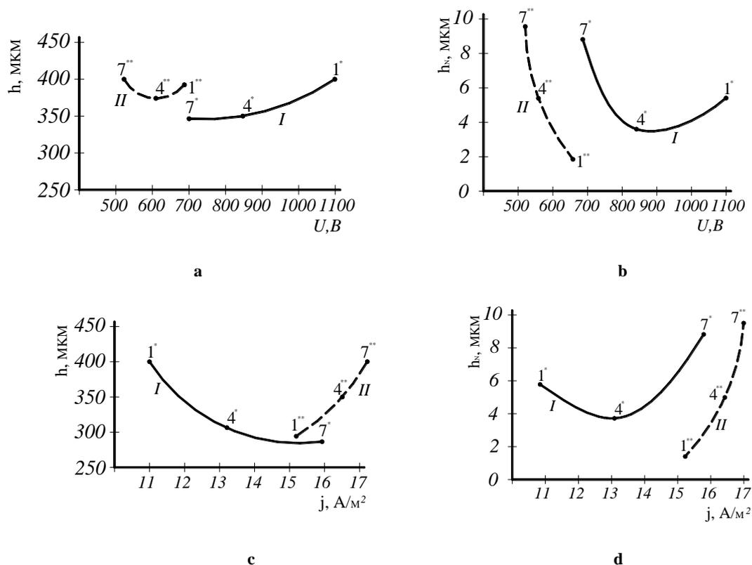
**Fig. 5. Dependences of the depths of the diffusion sphere  $h$  (a) and the nitride zone (b) on the voltage value  $U$ ; also (c, d) on the value of the current density  $j$  (I and II are different forms of suspensions) with the interdependent characteristics of the BATR**
