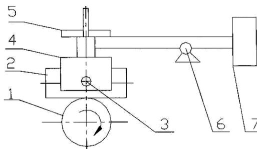
**Fig. 1. Scheme of the device for tests on wear according to the scheme of cross cylinders:
