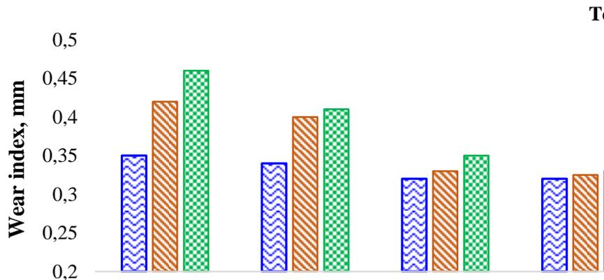
Fig. 3. Change in the wear index with an increase in the duration of the friction process in the turbine fuel Jet A-1: without additive (0) and at three different concentrations of FLNs (1, 2 and  $5 \cdot 10^{-4}$ , % wt.)
