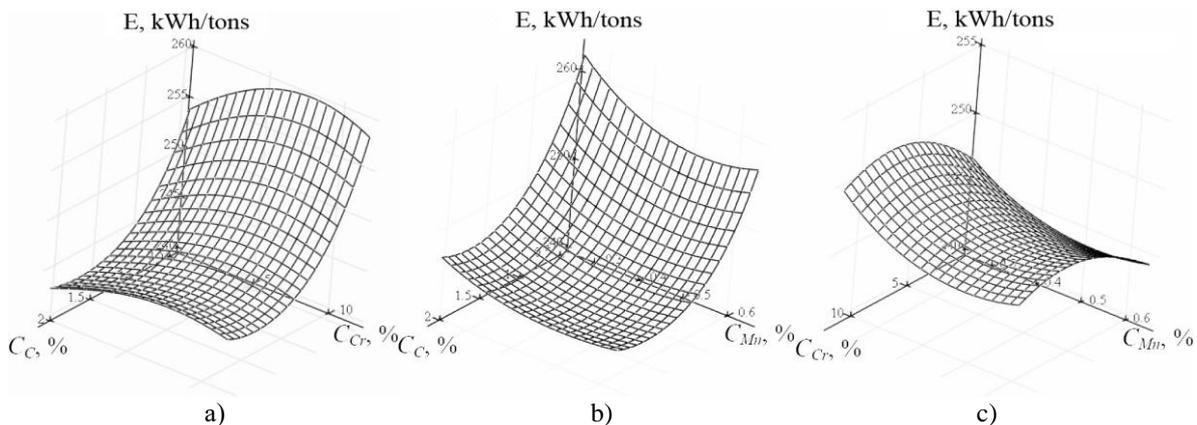
**Fig. 2. Response surfaces of the objective function - energy consumption  $E$  of the process of dehydration of the hardened screw press of mixed solid household waste in the planes of the parameters of impact after its operation and wear on the way  $s = 56850$  m (a) –  $E = f(C_C, C_{Cr})$ , (b) –  $E = f(C_C, C_{Mn})$ , (c) –  $E = f(C_{Cr}, C_{Mn})$**
