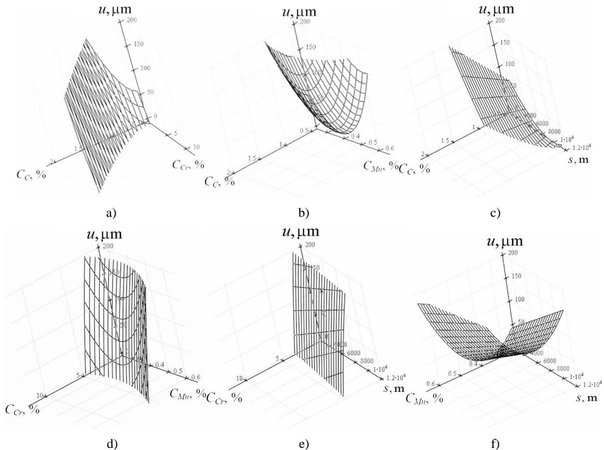
**Fig. 1. The response surfaces of the objective function - wear of the hardened auger  $u$  in the planes of the impact parameters (a) –  $u = f(C_C, C_{Cr})$ , (b) –  $u = f(C_C, C_{Mn})$ , (c) –  $u = f(C_C, s)$ , (d) –  $u = f(C_{Cr}, C_{Mn})$ , (e) –  $u = f(C_{Cr}, s)$ , (f) –  $u = f(C_{Mn}, s)$**
