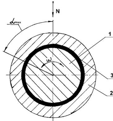
Fig. 4. Scheme of tribocoupling of parts in the oscillation mode: 1 – shaft; 2 – sleeve; 3 – coating.
