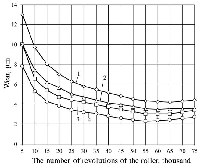
**Fig. 7. Dependence of the amount of wear of the "roller-pad" tribocoupling surfaces at the limit friction depending on the duration of the test ( $P = 1.5$  MPa,  $V = 0.5$  m/s). Tribocoupling of materials: 1 – "cast iron-PC", 2 – "cast iron-PCC", 3 – "steel-PC", 4 – "steel-PCC".**
