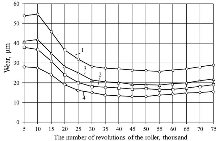
**Fig. 6. Dependence of the amount of wear of tribo-coupling friction surfaces of "roller-pad" samples without lubrication depending on the duration of the test ( $P = 1.5$  MPa,  $V = 0.5$  m/s). Tribocoupling of materials: 1 – "cast iron-PC", 2 – "cast iron-PCC", 3 – "steel-PC", 4 – "steel-PCC".**
