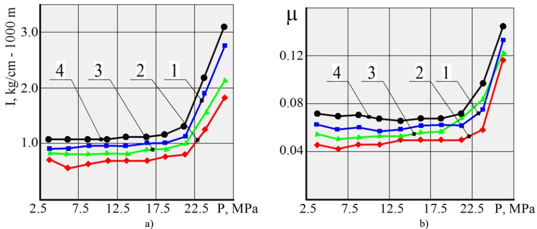
**Fig. 3. Dependence of wear intensity  $I$  (a) and friction coefficient  $\mu$  (b) of IN treatment on specific load  $P$  at sliding speed  $V$ :
