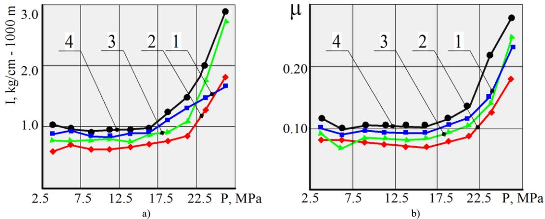
**Fig. 4. Dependence of wear intensity  $I$  (a) and friction coefficient  $\mu$  (b) of HT treatment on specific load  $P$  at sliding speed  $V$ : 1 –  $V = 0,4$  m/s; 2 –  $V = 0,7$  m/s; 3 –  $V = 1,0$  m/s; 4 –  $V = 1,3$  m/s**
