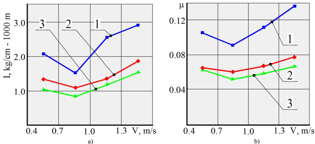
**Fig. 5. Dependence of wear intensity  $I$  (a) and friction coefficient  $\mu$  (b) on sliding speed  $V$  at specific load  $P = 20$  MPa and following treatment: 1 – HT; 2 – IN; 3 – HT+IN**
