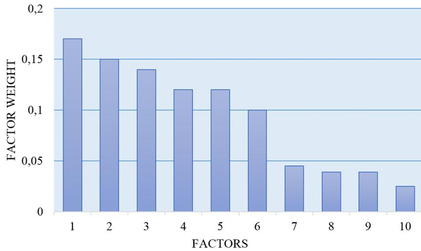
**Fig. 1. A ranked row of structural, technological and operational factors: 1 – saturation temperature; 2 – reactive gas pressure; 3 – composition of reactive gas; 4 – ion treatment time; 5 – operational load; 6 – sliding speed; 7 – coating thickness; 8 – part material; 9 – operating current of the saturation process; 10 – operating voltage of the saturation process**
