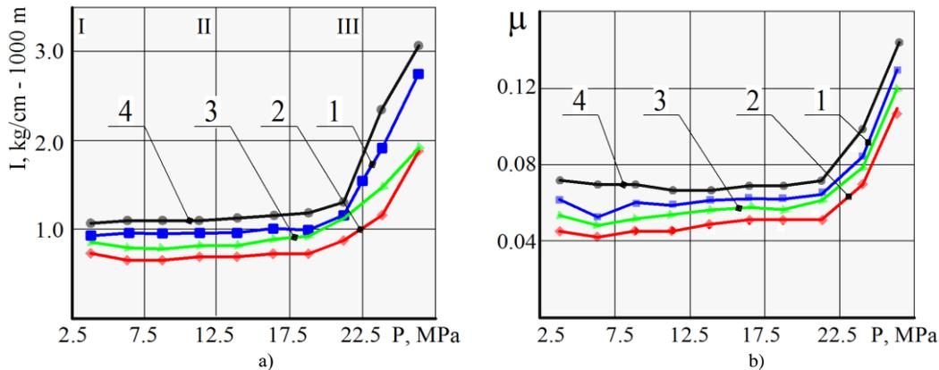
**Fig. 2. Dependence of wear intensity  $I$  (a) and friction coefficient  $\mu$  (b) of HT+IN treatment on specific load  $P$  at sliding speed  $V$ : 1 –  $V = 0.4$  m/s; 2 –  $V = 0.7$  m/s; 3 –  $V = 1.0$  m/s; 4 –  $V = 1.3$  m/s
