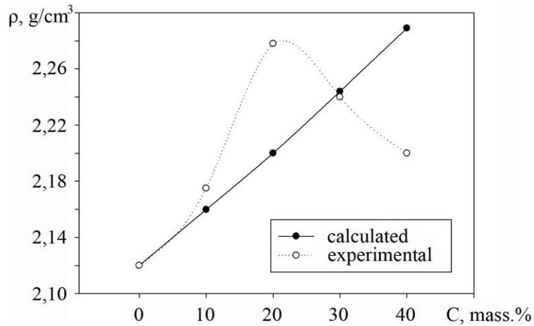
**Fig. 2.** Dependence of calculated and experimental density ( $\rho$ , g/cm<sup>3</sup>) of polytetrafluoroethylene on basalt fiber content (C, mass.%)
