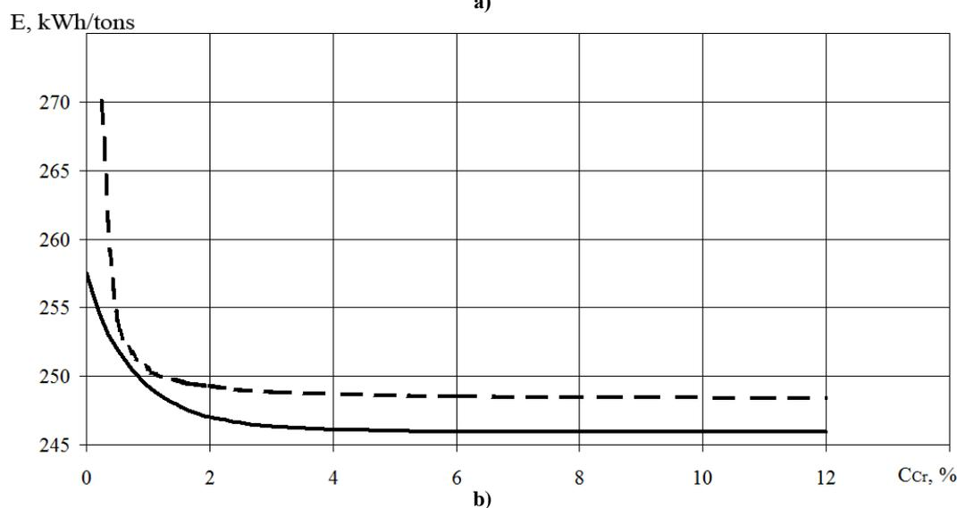
Fig. 2. The influence of an increase in the content of alloying elements in the steel of the auger after tempering on the energy intensity of the solid waste dehydration process after its operation and wear on the path  $s = 56850$  m (a) – manganese, (b) – chromium
