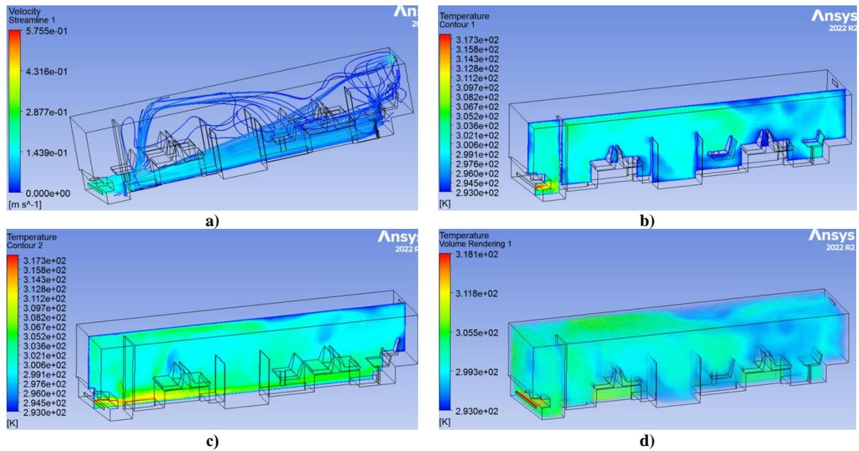
**Fig. 3. Velocity and temperatures distribution in the interior with a front layout: a) velocity in the interior; b) temperature distribution along the plane at the level of the left row of seats; c) temperature distribution along the plane at the level of the middle of the interior; d) temperature maps of the interior volume**
