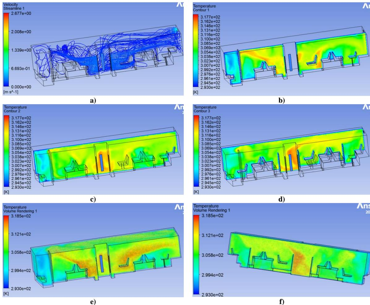
**Fig. 4. Velocity and temperature distribution in the interior with a middle vertically layout: a) velocity in the interior; b) temperature distribution along the plane at the level of the left row of seats; c) temperature distribution along the plane at the level of the middle of the interior; d) temperature distribution on the plane at the level of the right row of the interior; e), f) temperature maps of the interior volume**
