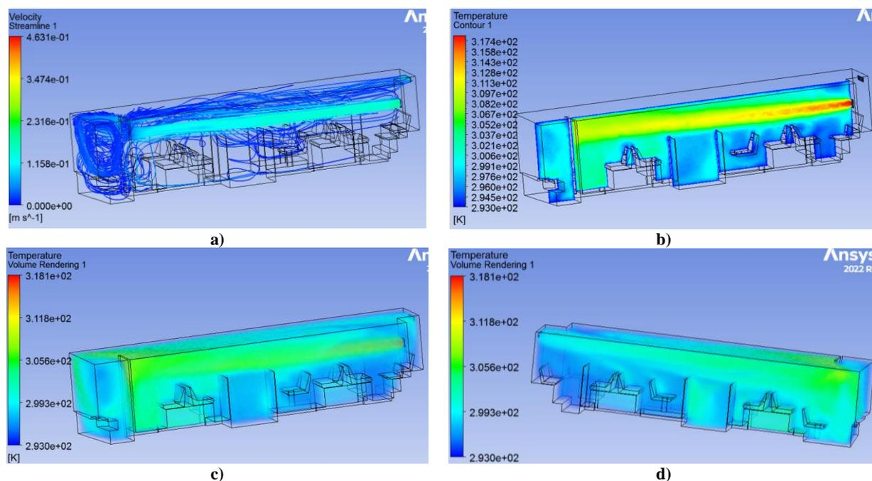
**Fig. 6. Velocity and temperature distribution in the interior with rear vertically shifted to the left layout: a) velocity in the interior; b) temperature distribution along the plane at the level of the left row of seats; c), d) temperature maps of the interior volume**
