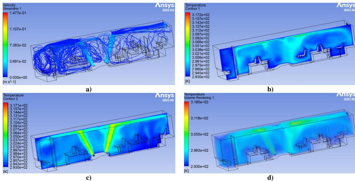
**Fig. 5. Velocity and temperature distribution in the interior for middle horizontally with an opposite engine layout: a) velocity in the interior; b) temperature distribution along the plane at the level of the left row of seats; c) temperature distribution along the plane at the level of the middle of the interior; d) temperature maps of the interior volume**
