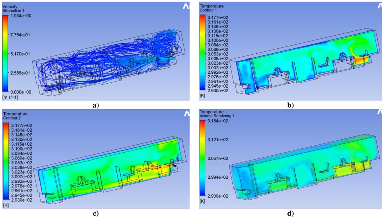
**Fig. 7. Velocity and temperature distribution in the interior for rear horizontally with an opposed engine layout: a) velocity in the interior; b) temperature distribution along the plane at the level of the left row of seats; c) temperature distribution along the plane at the level of the middle; d) temperature maps of the interior volume**
