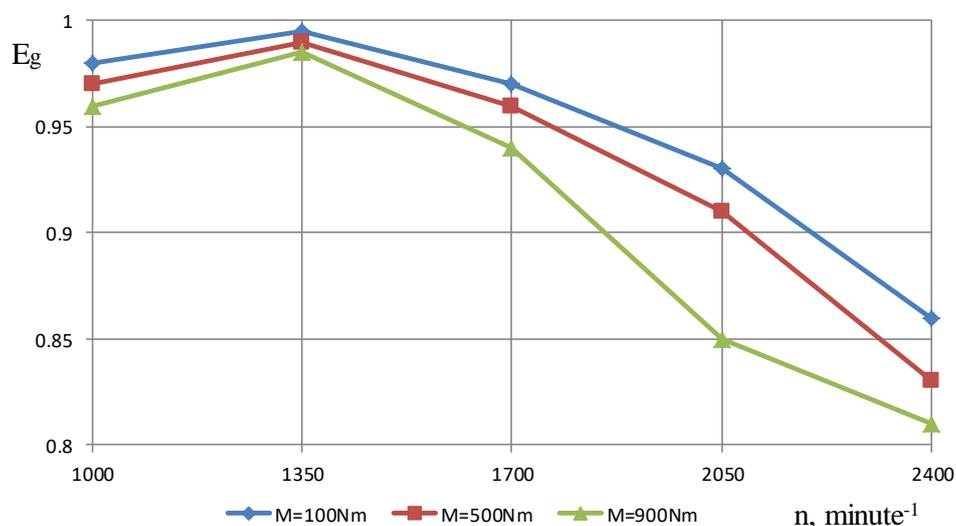
Fig. 5. Motor speed characteristics by parameter  $E_g$  ( $n$ )
