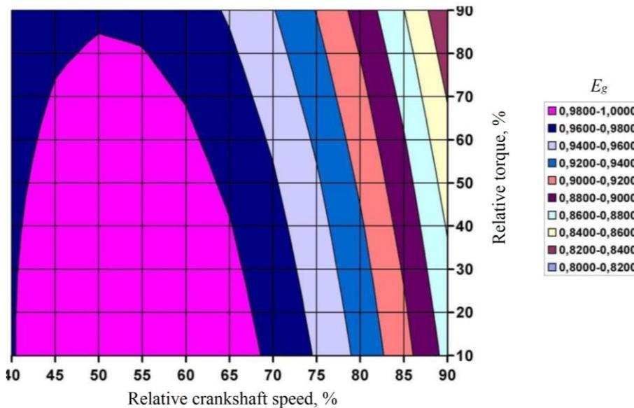
Fig. 8. Areas of parameter levels  $E_g$  in the field of the load-speed mode of the KamAZ engine
