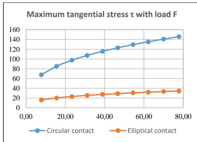
**Fig. 6. Effect of microgeometry in the point contact zone on the change in tangential stress  $\tau$  for friction bearing units with increasing load F**
