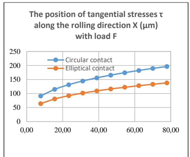
**Fig. 8. Influence of microgeometry on the position of penetration of tangential stresses  $\tau$  in the subsurface zone of point contact along the rolling direction  $x$  - ( $\mu\text{m}$ ) for friction bearing units with increasing load  $F$**
