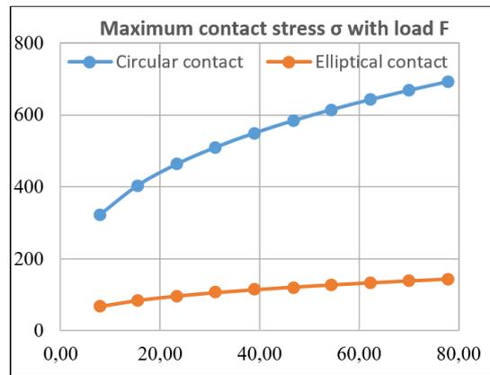
**Fig. 5. Influence of microgeometry in the point contact zone on the change in contact stress  $\sigma$  for friction bearing units with increasing load F**
