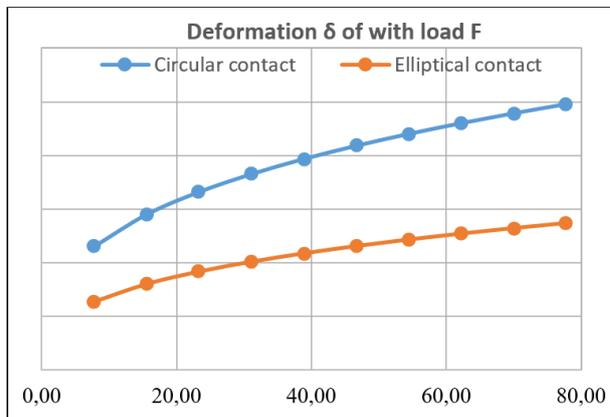
**Fig. 4. Influence of microgeometry in the point contact zone on the deformation  $\delta$  of contacting friction surfaces of bearing units with increasing load F**
