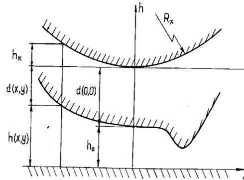
**Fig. 3. Microgeometry of circular friction contact taking into account elastic deformations:**
