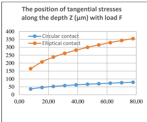
**Fig. 7. Influence of microgeometry on the position of penetration of tangential stresses  $\tau$  in the subsurface zone of point contact along the depth  $z$  - ( $\mu\text{m}$ ) for friction bearing units with increasing load  $F$**
