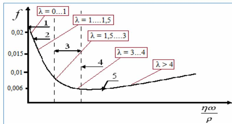
Fig. 5. Friction coefficient ( $f$ ) and lubrication mode ( $\lambda$ ) according to the Hersey-Striebeck diagram: 1 - dry, 2 - marginal, 3 - mixed; 4 - elastohydrodynamic; 5 - hydrodynamic lubrication modes.
