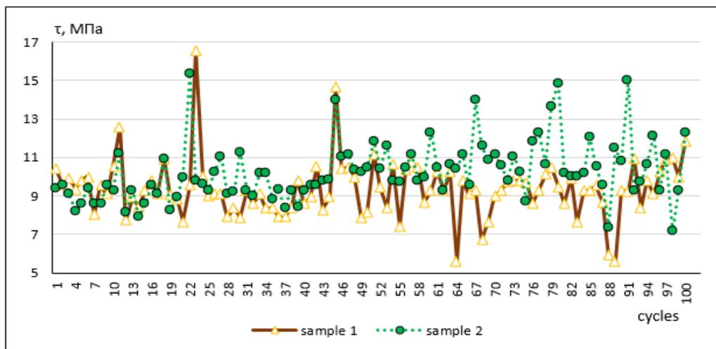
**Fig. 3. Kinetics of changes in shear stress of the lubricating layer in contact (τ).**
