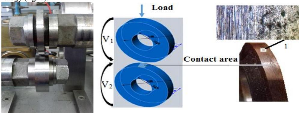
**Fig. 2. The diagram of the loading node of the test samples with rotation at speeds  $V_1$  and  $V_2$  and the appearance of the friction tracks of the 30ChGSA steel sample; 1 – section of the contact surface of the sample.**
