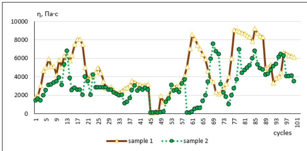
Fig. 4. Kinetics of changes in the effective oil viscosity ( $\eta$ ) in contact.
