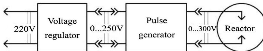
Fig. 2. Structural diagram of the EED installation
