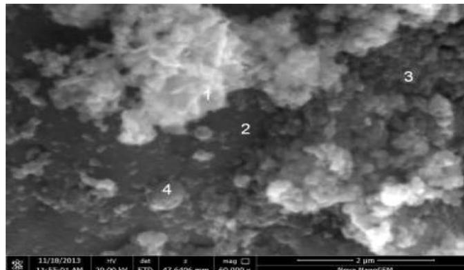
Fig. 5. Points of X-ray spectral microanalysis of powder
