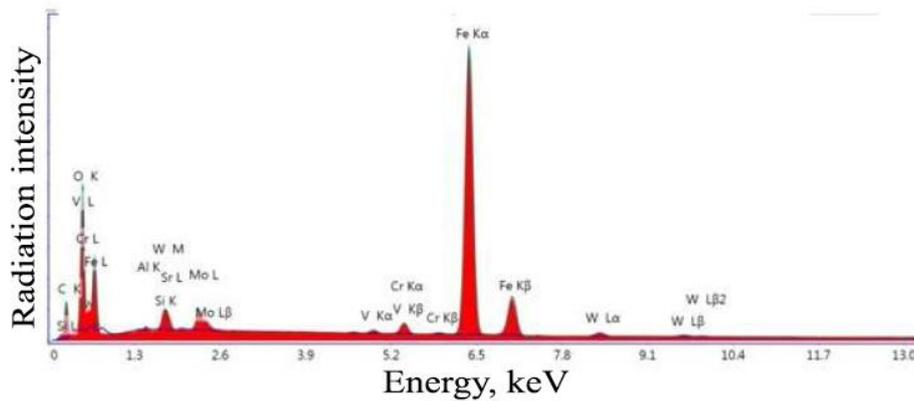
Fig. 6. X-ray spectral microanalysis of P6M5 powder at point 1
