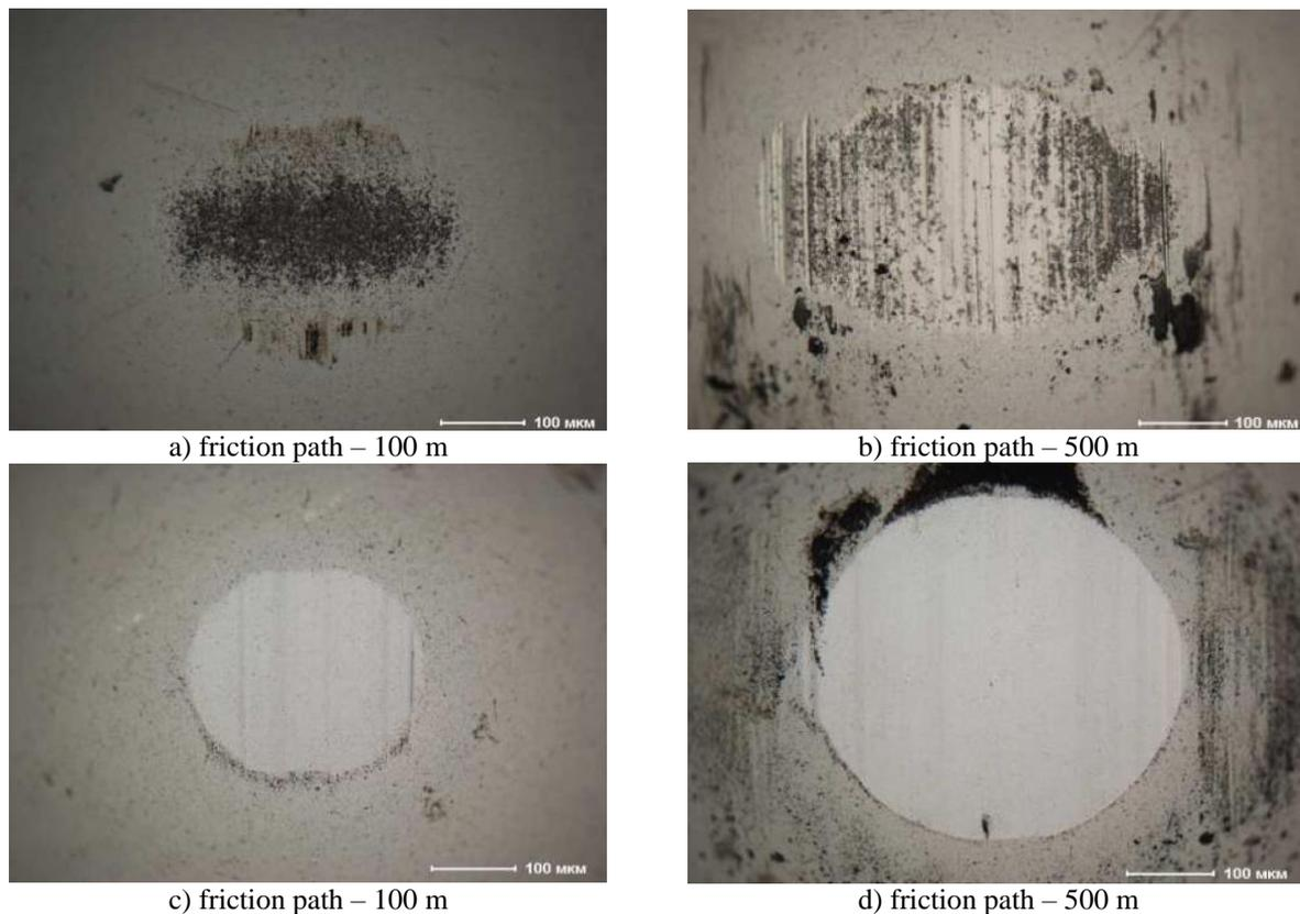
**Fig. 8. Optical image of the wear spot of the counterbody (ball) after passes over the investigated surface of the experimental samples: electrospark coatings from BRS (a, b); substrates made of steel 30KHSA (c, d)**
