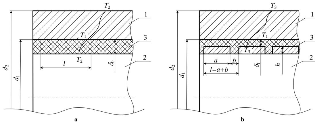
Fig. 1. Scheme of tribocoupling of parts "shaft-sleeve with polymer (a) and combined polymer-metal (b) coatings: 1 - sleeve; 2 - shaft; 3 - coating
