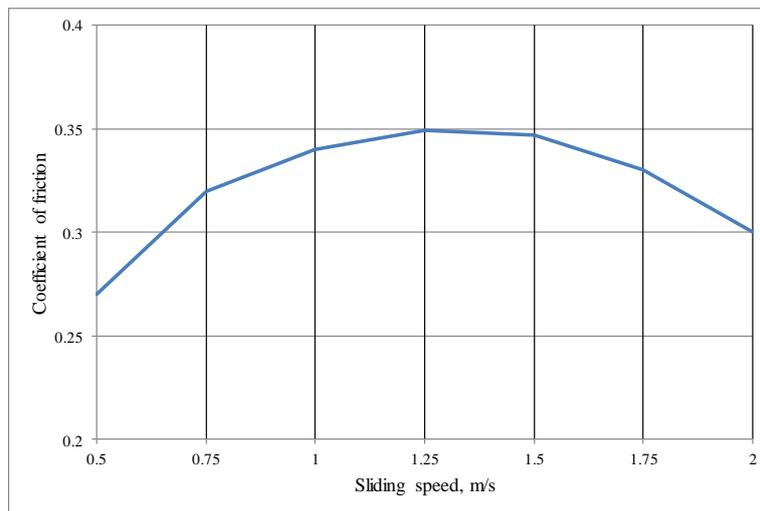
Fig. 4. Theoretical dependence of the PMeC friction coefficient on the sliding speed during friction without lubrication
