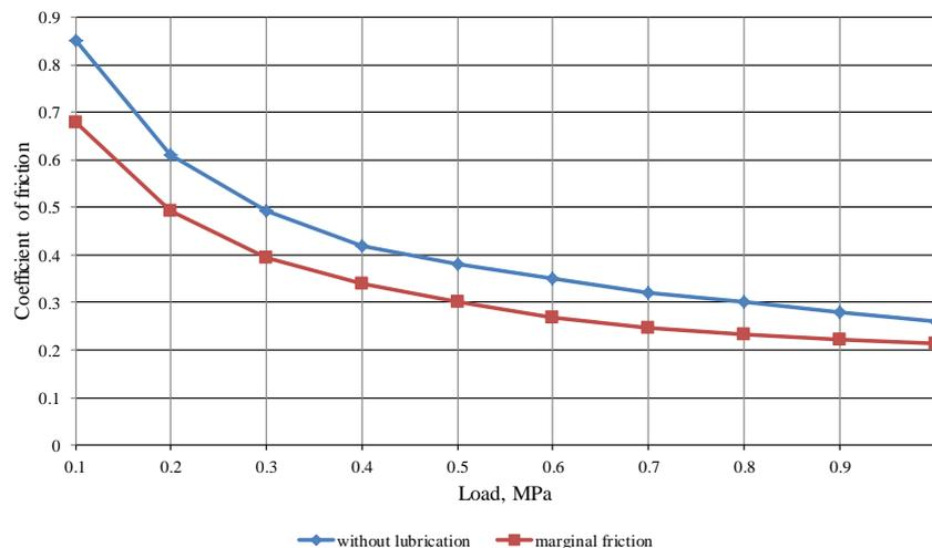
**Fig. 2. Theoretical curves of the dependence of the coefficient of friction of the polymer coating (PC) on the specific load**
