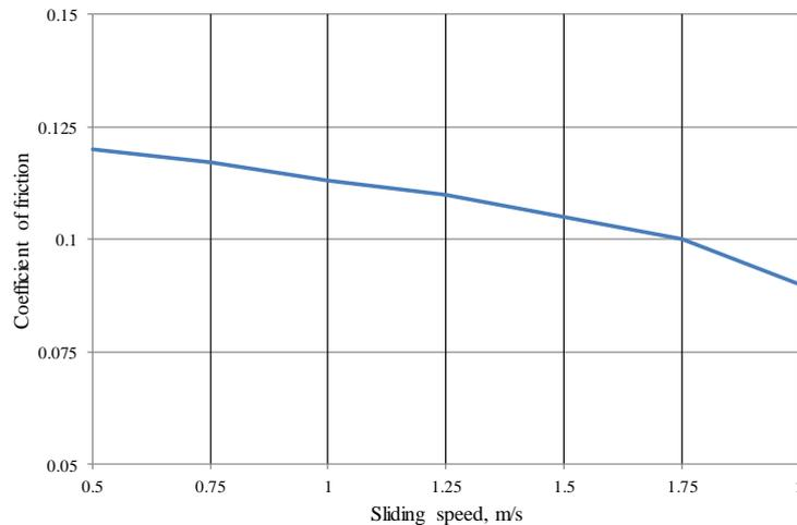
Fig. 5. Theoretical dependence of the PMeC friction coefficient on the sliding speed at the limit of friction
