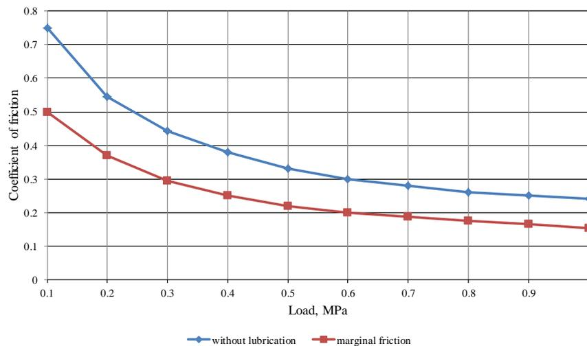
Fig. 3. Theoretical curves of the dependence of the coefficient of friction of the combined polymer-metal material (PMeC) on the specific load
