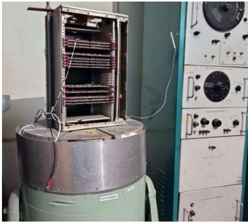
Fig. 3. Shaker VEDS-200 with a test electronic unit
