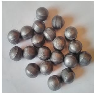
Fig. 2. General view of sintered ceramic ball blanks
