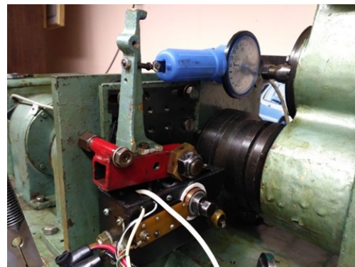
Fig. 3. Pad-roller tribopair at the SMC-2
