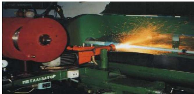
**Fig. 1. The electric arc spraying process**
