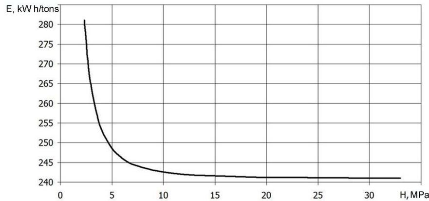
**Fig. 2. The influence of the microhardness of the auger coating on the energy intensity of the municipal solid waste dehydration process after its operation and wear on the path  $s = 56850$  m**
