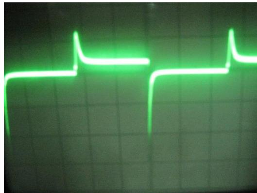
**Fig. 2. The shape of the change in the discharge current with a cyclically switched discharge of a rectangular shape with a slit  $\gamma = 2$ .**
