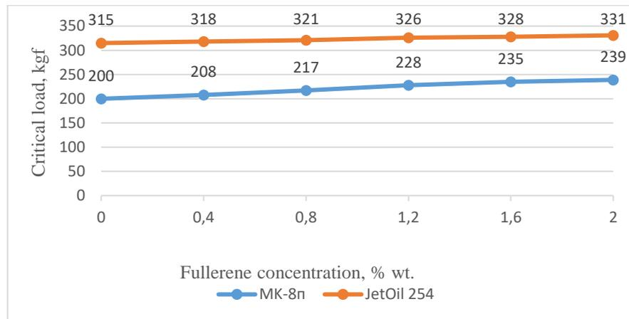
Fig. 5. Dependence of the critical load on the content of fullerene in the oil
