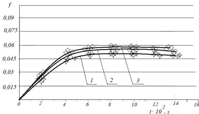
**Fig. 11.** Dependencies of the change in the friction coefficient during the tribosystem running-in for different load values  $N$ : 1 -  $N = 750$  N; 2 -  $N = 1500$  N; 3 -  $N = 2250$  N
