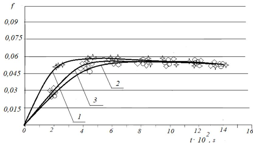
**Fig. 13. Dependencies of the change in the friction coefficient during tribosystem running-in for different sliding speed values  $v_{sl}$ : 1 –  $v_{sl} = 0,2 \text{ m/s}$ ; 2 –  $v_{sl} = 0,5 \text{ m/s}$ ; 3 –  $v_{sl} = 0,8 \text{ m/s}$**
