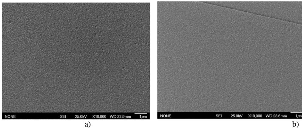
**Fig. 4. SEM-images of the Friction Surfaces of the Nanoscaled Detonation Coatings under the 0,2 MPa load (15 m/s) 10 000 zoom: a) 1 stripe area; b) 2 stripe area.**
