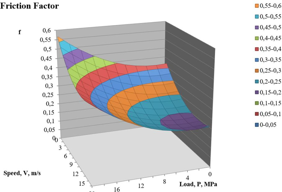
Fig. 2. Diagram of friction factor modeling of nanoscaled coating from friction speed and contact load.
