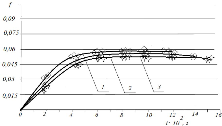
**Fig. 3. Dependencies of the change in the friction coefficient during the running-in of tribosystems with different form factors  $K_f$ : 1 –  $K_f=5 \text{ m}^{-1}$ ; 2 –  $K_f=12,5 \text{ m}^{-1}$ ; 3 –  $K_f=20 \text{ m}^{-1}$**
