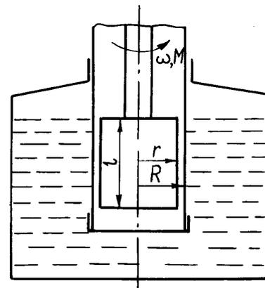
Fig. 2. Scheme of the coaxial-cylindrical system REOTEST 2.1.
