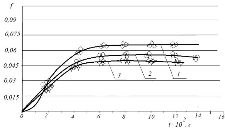
**Fig. 5. Dependences of the change in the friction coefficient during the run-in of tribosystems with different lubricating media  $E_u$ : 1 - hydraulic oil MG-15V ( $E_u = 2,43 \cdot 10^{14} \text{ J/m}^3$ ); 2 - motor oil M - 10G2κ ( $E_u = 3,6 \cdot 10^{14} \text{ J/m}^3$ ); 3 - transmission oil TSp-15κ ( $E_u = 4,18 \cdot 10^{14} \text{ J/m}^3$ )**
