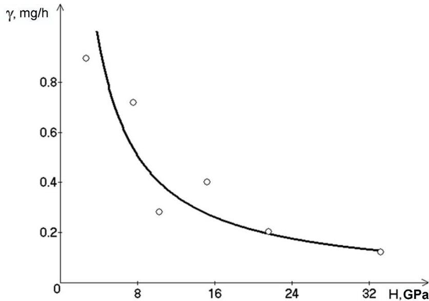
**Fig. 1. Dependence of the change in the auger wear rate depending on the microhardness of the coating: actual  $\circ$ , theoretical —**
