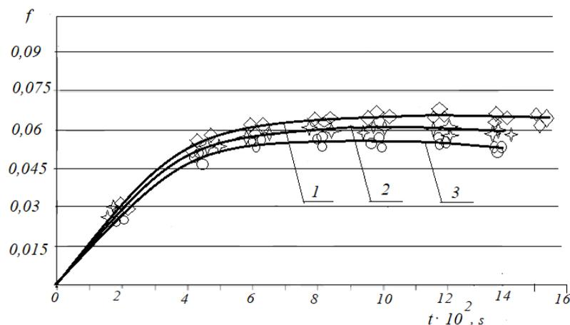
**Fig. 7. Dependences of the change in the friction coefficient during the running-in of tribosystems with different combined materials  $RS_{TS}$ : 1 - steel 40X + steel 40X, ( $RS_{TS} = 249,9 \text{ m}^{-1}$ ); 2 - steel 40X + VCh 70, ( $RS_{TS} = 309 \text{ m}^{-1}$ ); 3 - steel 40X + Br.AZH 9-4, ( $RS_{TS} = 332,5 \text{ m}^{-1}$ )**
