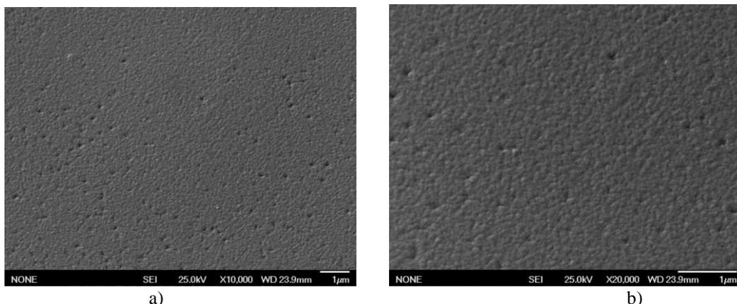
Fig. 3. SEM-images of the Initial Surfaces of the Nanoscaled Detonation Coatings: a) 10 000 zoom; b) 20 000 zoom.
