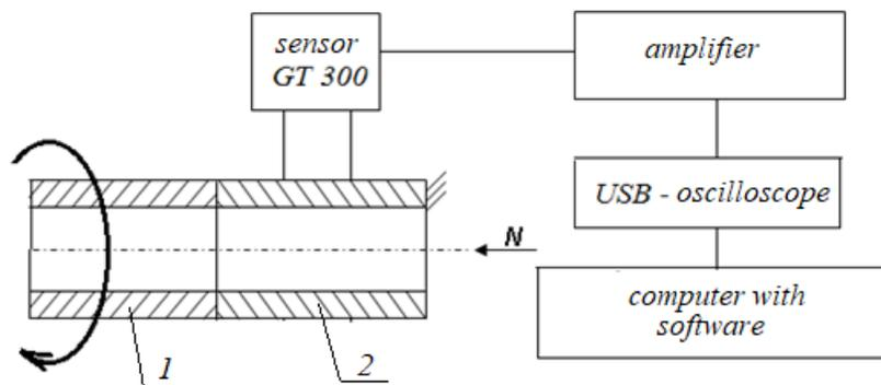
**Fig. 1. Block diagram of the experimental equipment for registration and processing of AE signals: 1 - moving triboelement; 2 - fixed triboelement; N - load**
