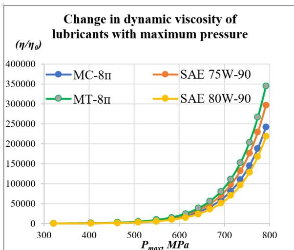
Fig. 3. Influence of the rheological feature (change in dynamic viscosity) of lubricants of different physical and chemical composition with increasing maximum pressure, taking into account the temperature in the contact zone  $T = 343 \text{ K}$  for friction bearing units
