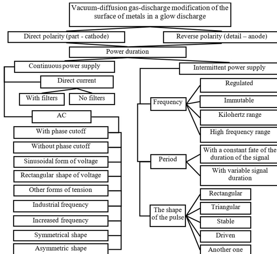
**Fig. 1. Classification of nitriding processes in glow discharge according to the criterion of power source characteristics**
