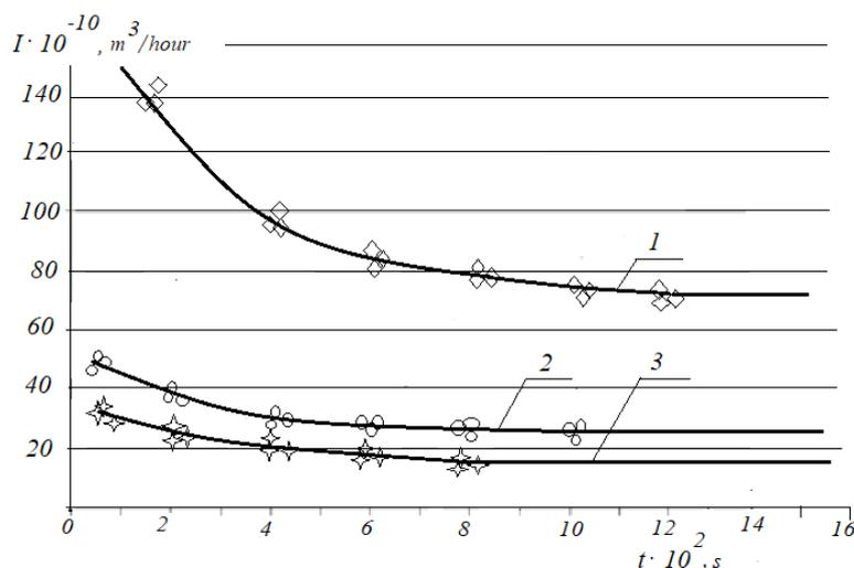
**Fig. 4. Dependencies of changes in the volumetric rate of wear during the running-in of tribosystems with different lubricating media  $E_u$ : 1 - hydraulic oil MG–15V ( $E_u = 2,43 \cdot 10^{14} \text{ J/m}^3$ ); 2 - motor oil M – 10G<sub>2κ</sub> ( $E_u = 3,6 \cdot 10^{14} \text{ J/m}^3$ ); 3 - transmission oil TSp-15κ ( $E_u = 4,18 \cdot 10^{14} \text{ J/m}^3$ )**
