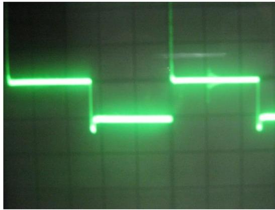
**Fig. 3. The shape of the discharge voltage change with a CSD of a rectangular shape with a slit  $\gamma = 2$ .**
