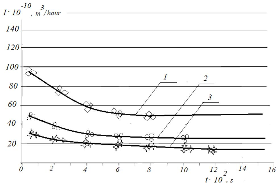
Fig. 2. Dependences of changes in the volume rate of wear during the running-in of tribosystems with different shape factors  $K_f$ : 1 –  $K_f = 5 \text{ m}^{-1}$ ; 2 –  $K_f = 12,5 \text{ m}^{-1}$ ; 3 –  $K_f = 20 \text{ m}^{-1}$
