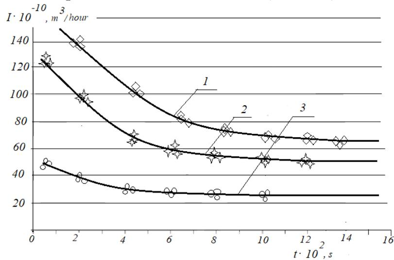
**Fig. 6. Dependences of the change in the volumetric rate of wear during the running-in of tribosystems with different composite materials  $RS_{TS}$ : 1 - steel 40X + steel 40X, ( $RS_{TS} = 249,9 \text{ m}^{-1}$ ); 2 - steel 40X + VCh 70, ( $RS_{TS} = 309 \text{ m}^{-1}$ ); 3 - steel 40X + Br.AZH 9-4, ( $RS_{TC} = 332,5 \text{ m}^{-1}$ )**
