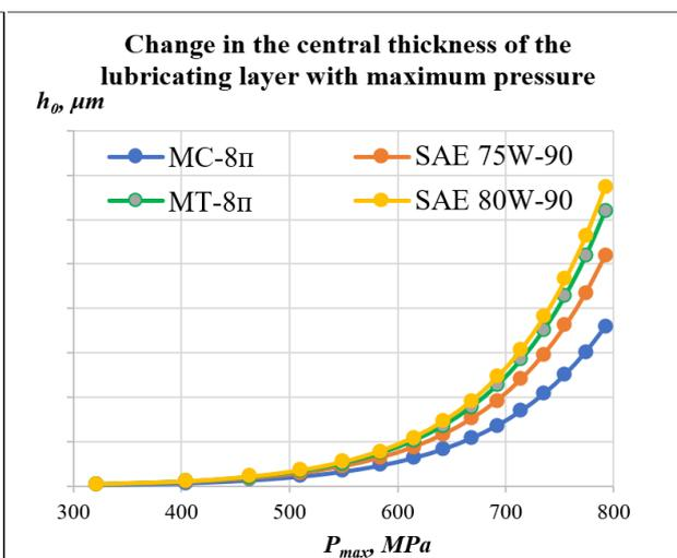
Fig. 4. Change in the central thickness of the lubricating layer with increasing maximum pressure, taking into account the temperature in the contact zone  $T = 343 \text{ K}$  for friction bearing units lubricated with lubricants of different physical and chemical composition
