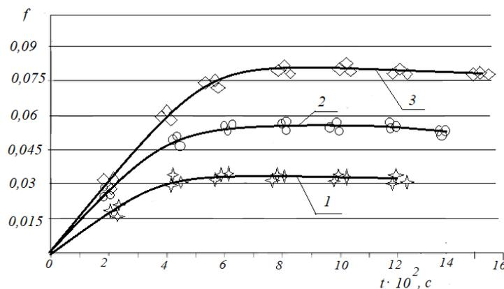
Fig. 9. Dependencies of the change in the friction coefficient during the running-in of tribosystems for different roughness values on the friction surfaces  $Ra$ : 1 –  $Ra = 0,16$  micron; 2 –  $Ra = 0,2$  micron; 3 –  $Ra = 0,24$  micron
