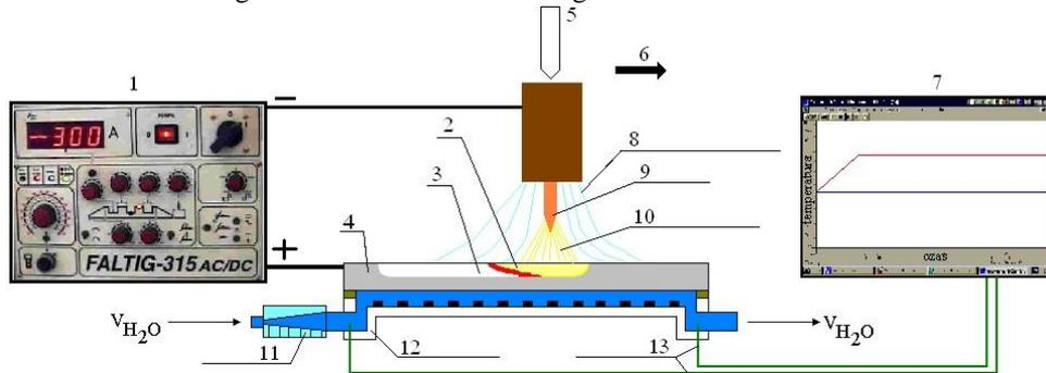
**Fig. 1. Schematic of the installation for melting and calorimetric studies (method GTAW: Gas-Tungsten-Arc-Welding):** 1 - current source, 2 - liquid metal welding bath, 3 - melted layer, 4 - sample, 5 - protective gas, 6 - direction of arc movement, 7 - temperature gauge, 8 - protective atmosphere, 9 - electrode, 10 - electric arc, 11 - flow meter, 12 - calorimeter, 13 - thermocouple
