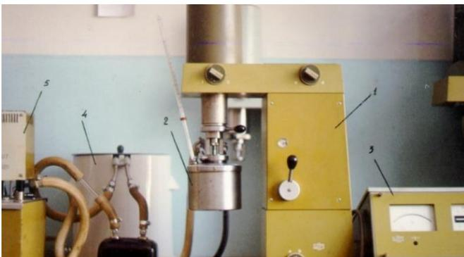
Fig. 1. General view of the rotational viscometer REOTEST 2.1.
