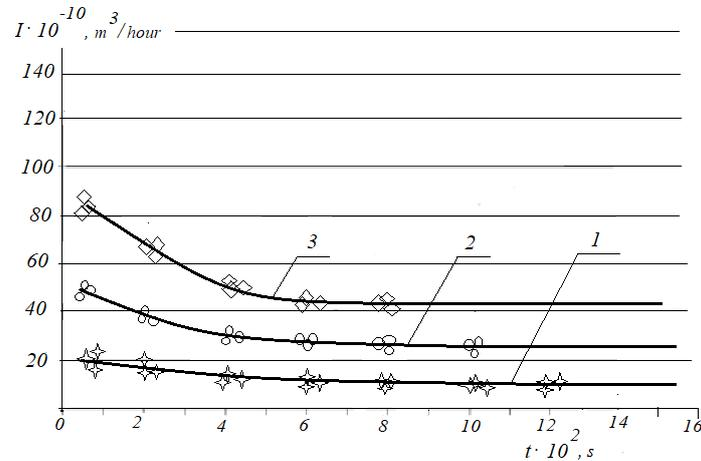
**Fig. 10.** Dependencies of the change in the volumetric rate of wear during tribosystem running-in for different load values  $N$ : 1 -  $N = 750$  N; 2 -  $N = 1500$  N; 3 -  $N = 2250$  N
