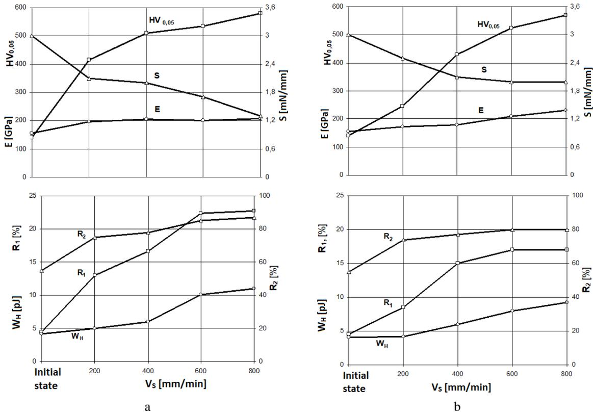
Fig. 7. Effect of arc scanning speed on the micromechanical properties of hardened surfaces at  $I = 100$  A (a) and  $I = 200$  A (b):  $HV_{0,05}$  – microhardness;  $E$  – Young's modulus of elasticity;  $S$  – contact rigidity;  $R_1$  and  $R_2$  – relaxation capacity in the first and second cycles;  $W_H$  – hysteresis loop area
