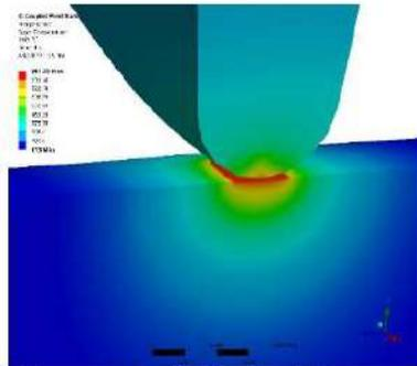
Fig. 5. Temperature distribution in the contact zone
