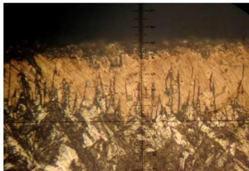
**Fig. 4. The microstructure of the diffusion borochrome layer on steel 30: temperature 1000°C, saturation time - 6 h (the price of the scale division is 5 μm)**
