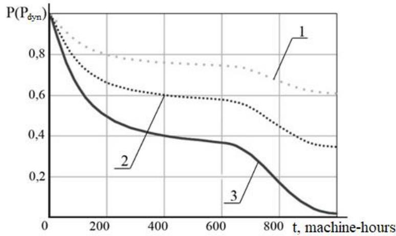
Fig. 3. категория Graph of changes in the probability of failure-free operation of a bulldozer blade  $P(P_{dyn})$  with the time of its operation in an abrasive environment  $t$ , h: 1 - I category of soil, 2 - II category, 3 - III category
