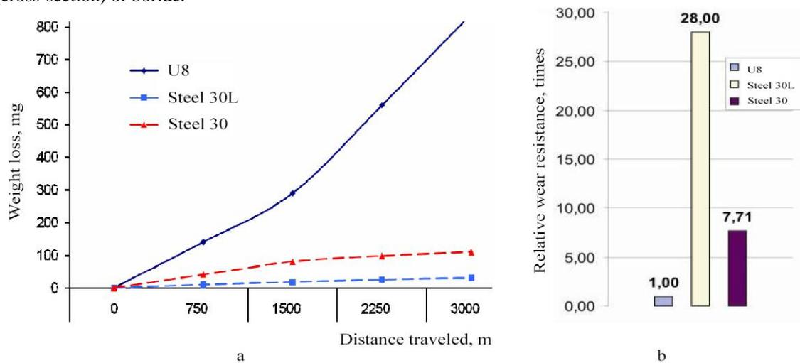
**Fig. 5. Wear resistance during abrasive wear of carbon steel (0.3% carbon): steel 30 - solid-phase boronization from coating, steel 30L - saturation of the surface with boron during LGM (a - mass loss, b - relative wear resistance)**
