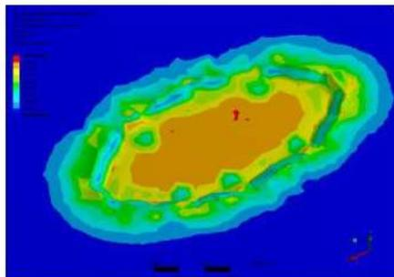
Figure 3.11 – Stress-strain state of the contact patch
