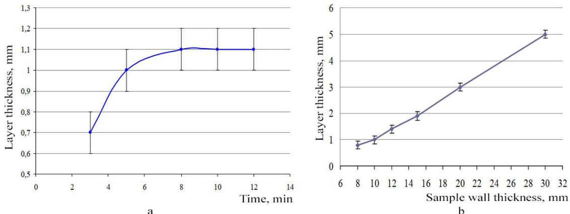
**Fig. 1. Effect on the thickness of the borochrome layer on 45L steel:**
