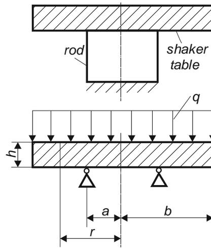
Fig. 2. Load scheme of the deformable shaker table by its own weight
