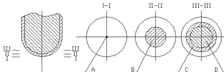
**Fig. 1. Stages of wear of the coated sample**
