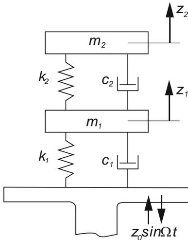
Fig. 1. Dynamic model of oscillations of an electronic product fixed on a rigid shaker table
