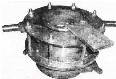
**Fig. 2. Current-driven crystallizer  $\varnothing 90\text{ mm}$**
