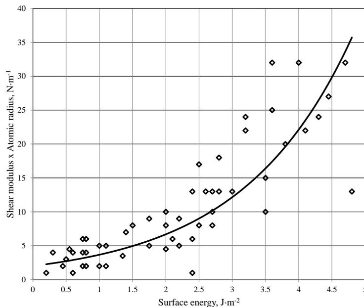
**Fig. 2. Correlation between the value of the macroscopic shear modulus per atomic radius and the surface energy of homogeneous contact materials**
