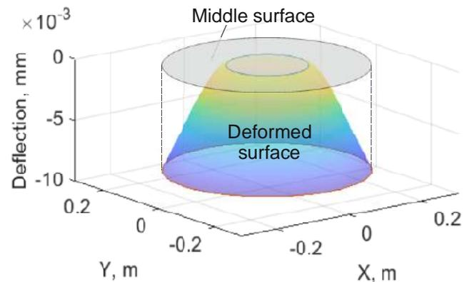
Fig. 4. Static deflection of the shaker table at absence of displacement
