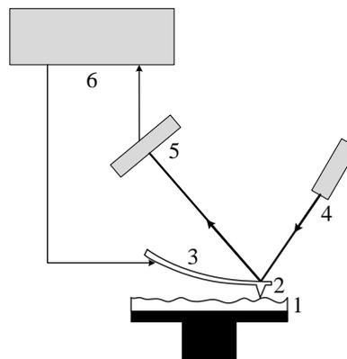
**Fig. 1. Block diagram of the principle of measurement of the examined surface in an atomic force microscope: 1 – the examined surface of the sample; 2 – probe (probe); 3 – cantilever; 4 – laser beam; 5 – photodiode; 6 – electronic conversion and feedback device**
