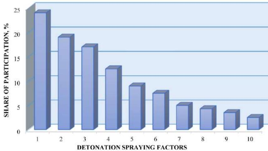
Fig. 1. Ranked series of detonation spraying factors: technological parameters (1 – powder material; 2 – base material; 3 – powder weight per cycle; 4 – spraying distance; 5 – volume of detonating mixture; 6 – number of shots per second; 7 – temperature of water for barrel cooling; 8 – speed of part movement), constructive parameters (9 – coating thickness; 10 – powder granulation).
