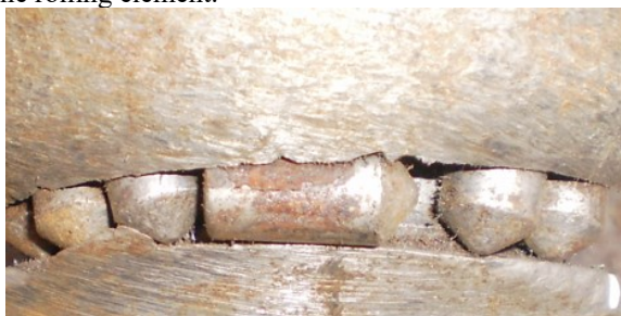
Fig. 1 Appearance of worn rollers of the bearing assembly after operation
