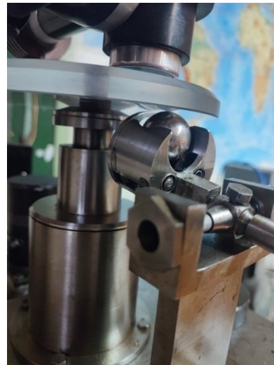
Fig. 2. Contacting pair: steel ball – glass disk
