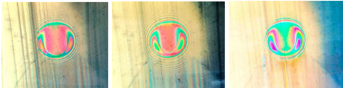
Fig. 6. Selection of micro-interferograms for point EHD contact ( R_y/R_x = 1 ) over a range of linear rolling velocity V from 0.05 to 1.0 m/s (SAE 80W-90 transmission oil)
