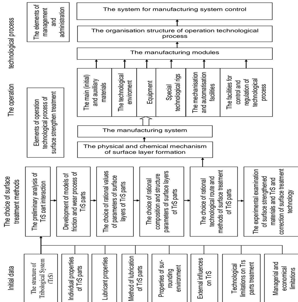
Fig. 1. Scheme of development of operation technology of surface strengthen treatment
