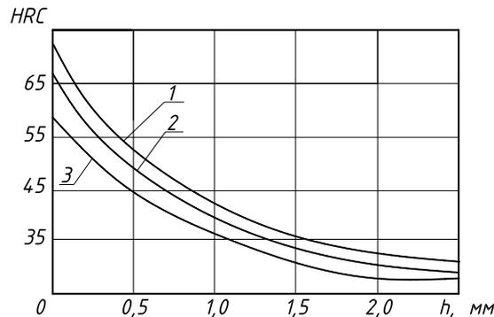
**Fig. 3. Changes in the hardness of the depth of the plowshares depending from the recovery method: 1 - restored by welding tires made of steel 45 with sormite surfacing and vibration hardening, 2 - new plowshares made of L-53 steel subjected to vibration hardening, 3 - new plowshares made of steel 65G, strengthened by vibration deformation**
