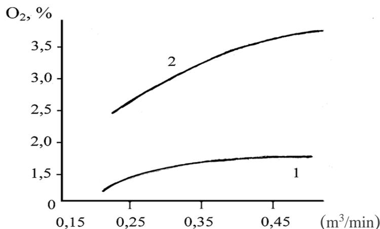
Fig. 2. The effect of the spraying air consumption on the amount of oxygen in the coatings obtained by gas-flame spraying in mode 1 (1) and electric arc spraying in mode 4 (2)
