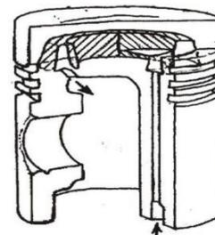
Fig. 2. The scheme of cooling the piston head
