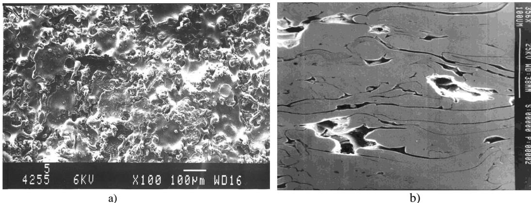
**Fig. 1. Microtopography (a) and microstructure (b) of steel gas-thermal coating**
