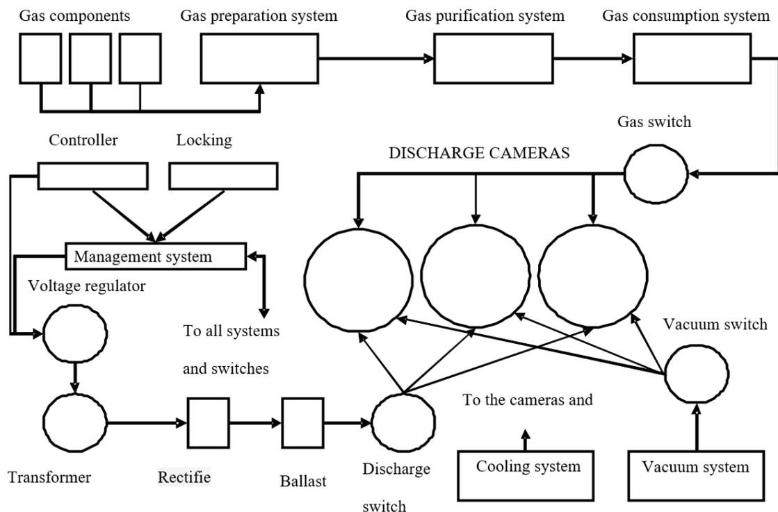
**Fig. 1. Block diagram of a three-chamber installation**
