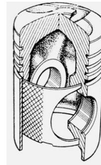
Fig. 6. Piston with thermostatic insert
