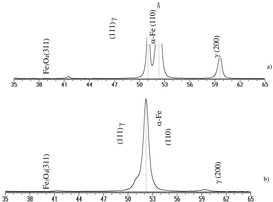
**Fig. 3. Fragments of X-ray diffraction patterns from the surface layers of coatings after gas-flame (a) and electric arc spraying (b)**
