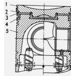
Fig. 4. Piston with heat pad and inseparable heat ring: 1 - head; 2 - inseparable heat ring; 3 - thermal insulation; 4 - ring holder; 5 - piston
