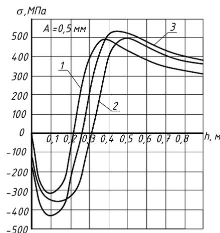
**Fig. 4. Changes in residual stresses in depth depending on the method of plowing recovery, amplitude of oscillations of the processing tool and processing time  $t = 20$  s: 1 - restored welded tires of steel 45 with surmaite surfacing and vibration hardening, 2 - new plowshares of steel L-53 subjected to vibration deformation, 3 - new plowshares made of steel 65G, strengthened by vibration deformation**
