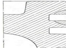
Fig. 16. Sealing of the upper groove of the piston by remelting by doping
