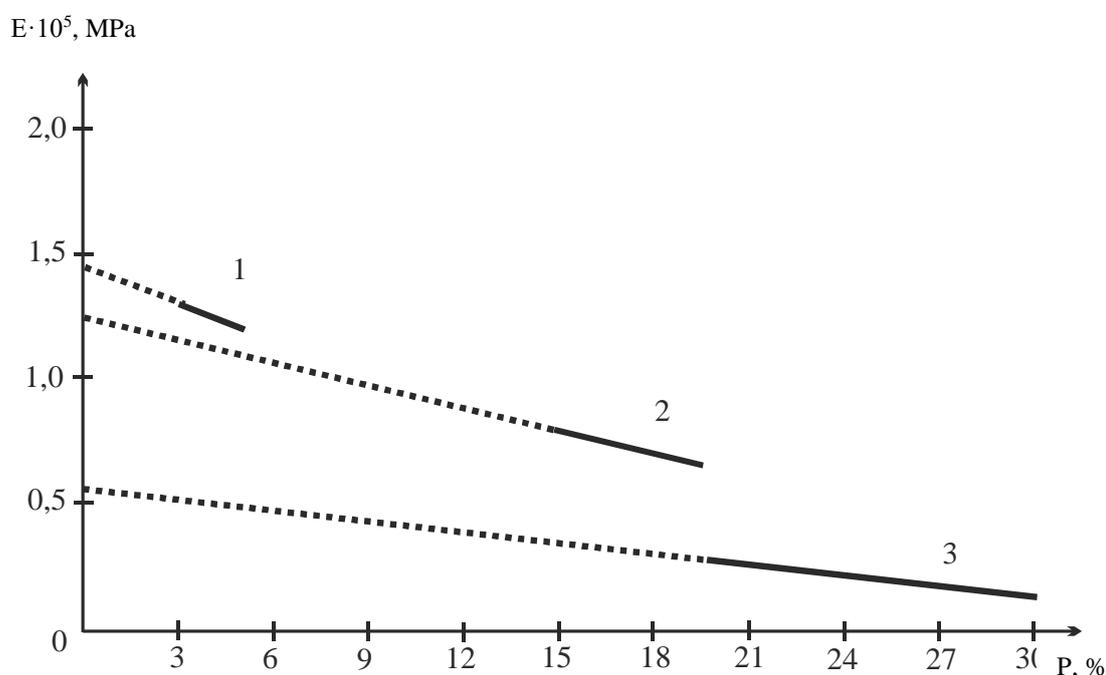
**Fig. 1. Relationship between porosity and elastic modulus of coatings: 1 – coating obtained by the electric contact method; 2 – coating obtained by electric arc spraying; 3 – coating obtained by the gas flame method**
