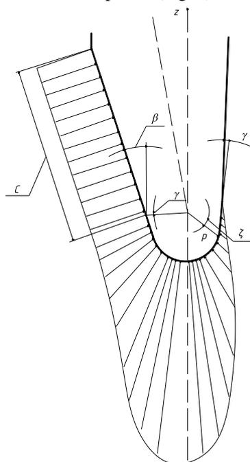
Fig. 1. Scheme of stress distribution in the cutting part of the ploughshare
