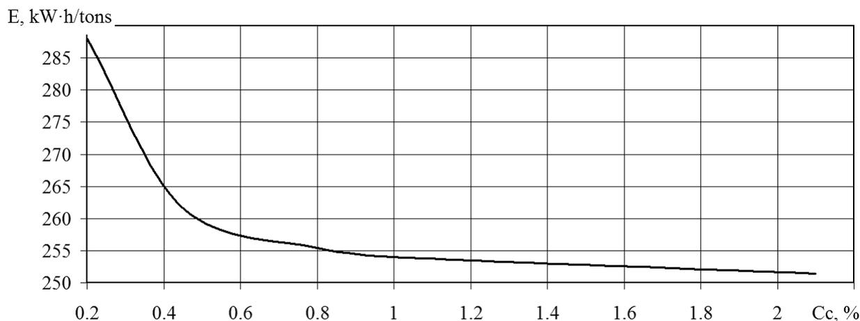
**Fig. 4.** The effect of increasing the carbon content in the auger material on reducing the growth rate of energy consumption of the dehydration process MSW after its two-week operation and wear ( $s = 56850$  m)
