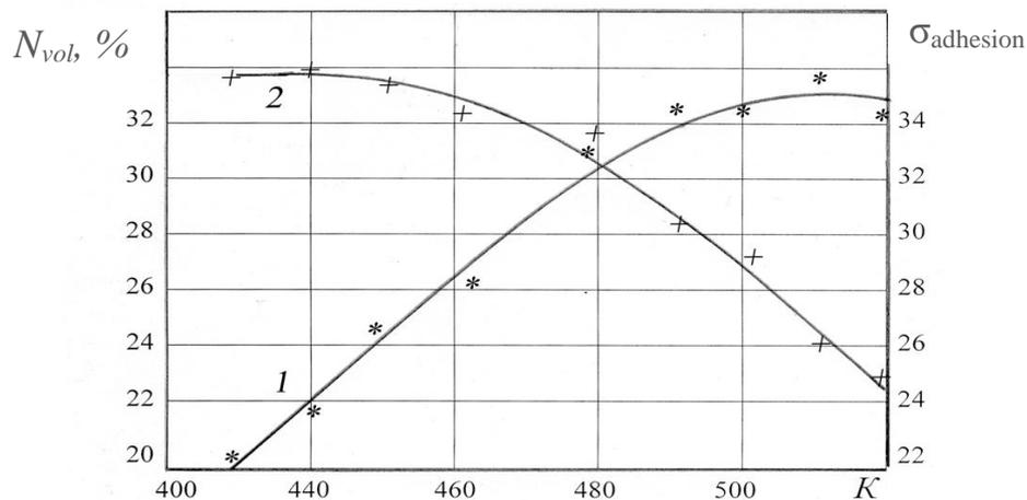
Fig. 4. The dependence of the amount of metastable austenite (vol.%) (1) in steel coatings 2Kh18N10T and 40KhN and their adhesion (MPa) (2) on the preheating temperature of the recoverable surface
