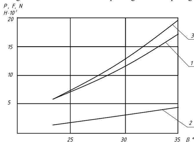
Fig. 2. Curves of changes of efforts on a blade depending on a sharpening angle:
