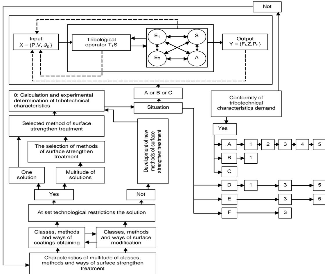
Fig. 2. Scheme of selection of optimal methods of surface strengthens treatment.
