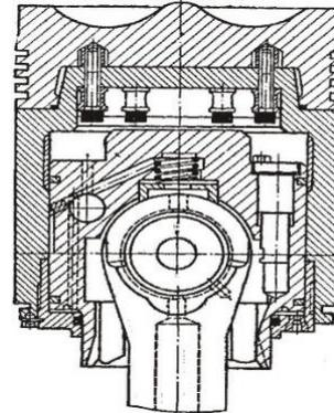
Fig. 9. Diesel piston with varying degrees of compression
