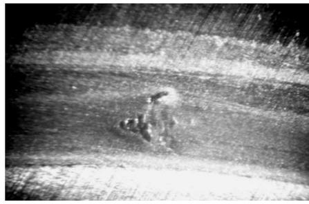
Friction track of a sample made of 40X steel, tempered and nitrided
