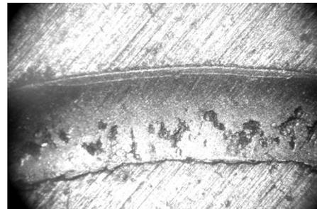
Friction track of a sample made of 40X steel without heat treatment
