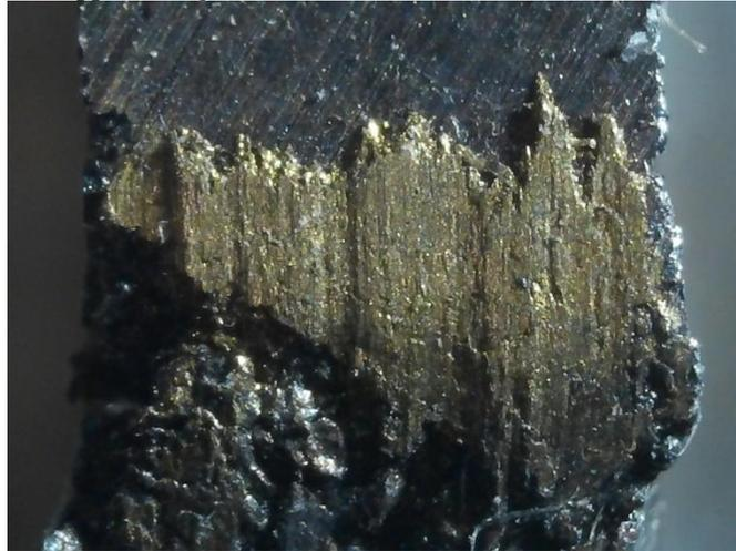
Fig. 11. The sticking of brass L63 on the rear surface of the cutter made of cast iron SCh20 when rubbing
